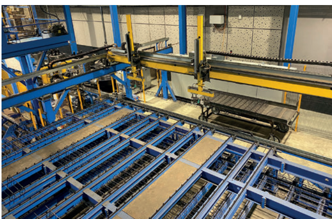
All manufactured lattice girders are placed on a buffer magazine by a crane robot, which then automatically and individually feeds them to the laying robot.
