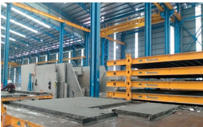
The solid slabs and walls are already equipped with reinforcement and ready for transport and installation on site.
