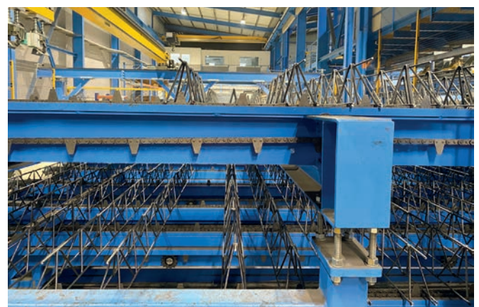
All manufactured lattice girders are placed on a buffer magazine by a crane robot, which then automatically and individually feeds them to the laying robot.
