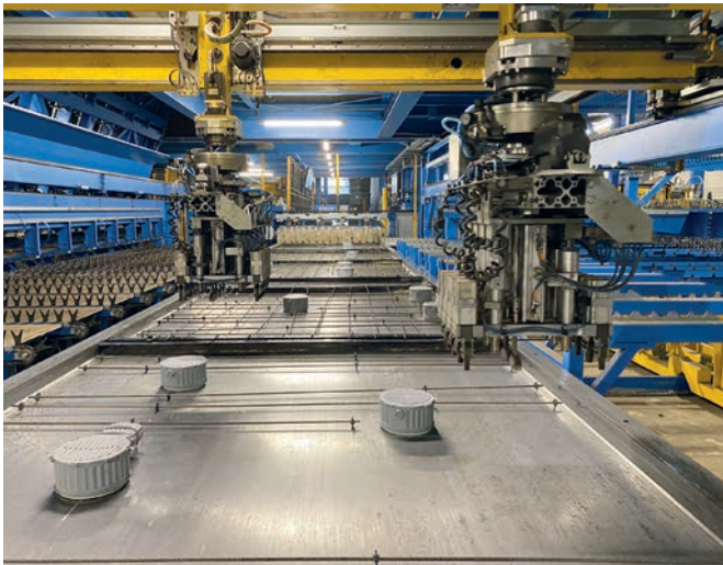
Multi-axis robot for placing the reinforcement
