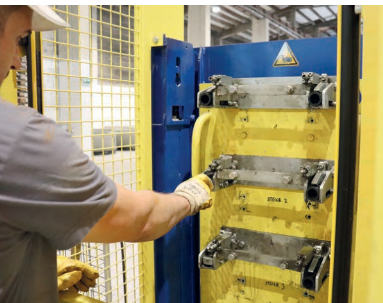
Insertion of sleeves for optional step pegs in the Stepmaster magazine
