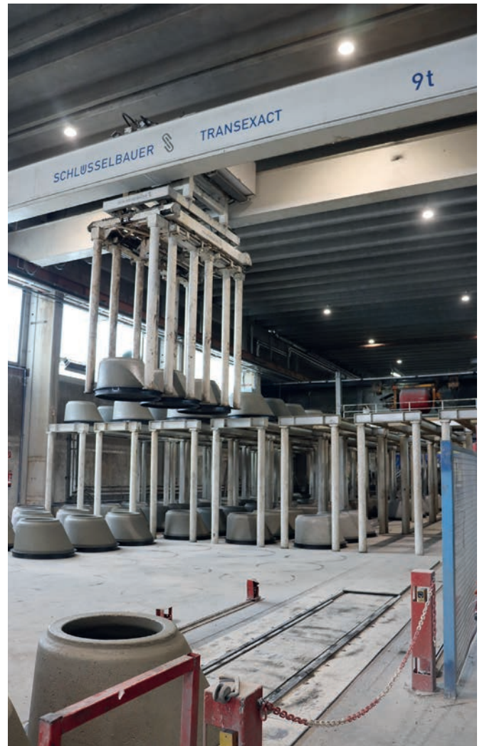
The modular, fully automatic Exact production system for pipes and manhole components has been in operation at Sollenau since 1998.
