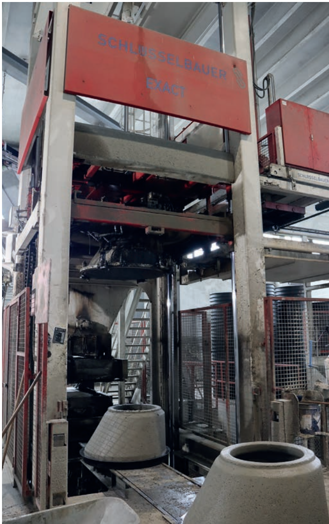
The modular, fully automatic Exact production system for pipes and manhole components has been in operation at Sollenau since 1998.
