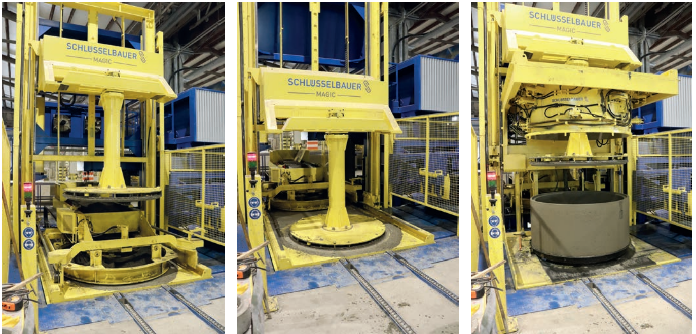
The filling of the Magic production system with concrete. The compaction process and the ejection of the finished product are fully automated.
