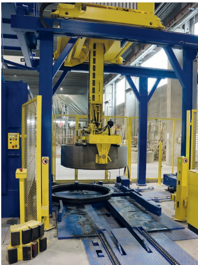
After the manipulator has lifted the manhole part and thus released it from the pallet, it is directly inserted into the cleaning station.
