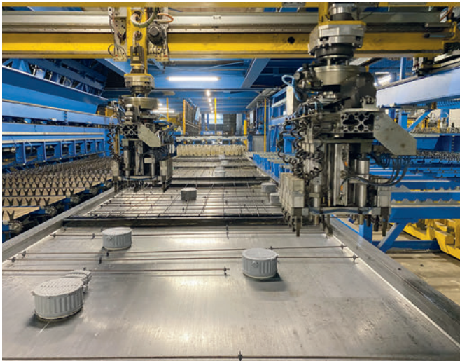
Multi-axis robot for placing the reinforcement
