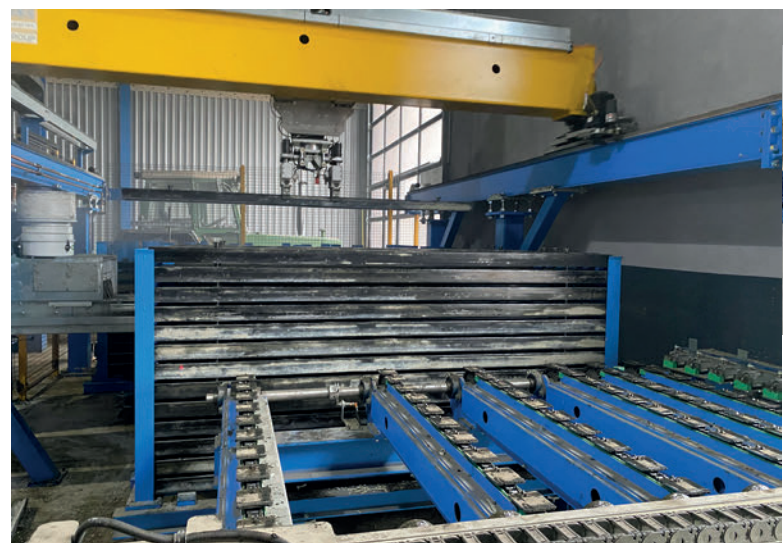
Storage robot in the active storage area
