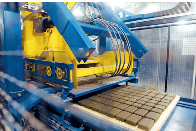
Masa concrete block making machine XL 9.1
