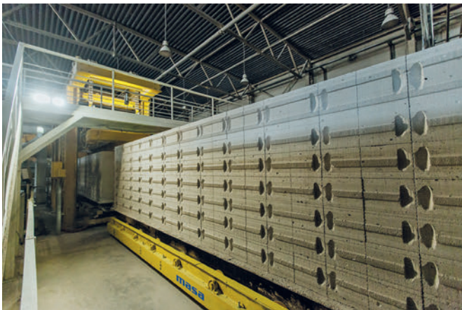
Production of sand lime bricks with the Masa hydraulic press HDP 800
