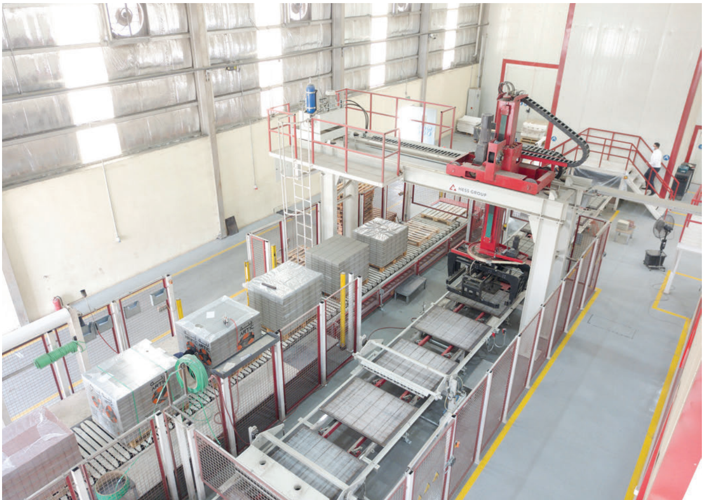
The packets of blocks are formed on the 28-m long slat conveyor arranged in parallel and then transported outdoors in cycles.
