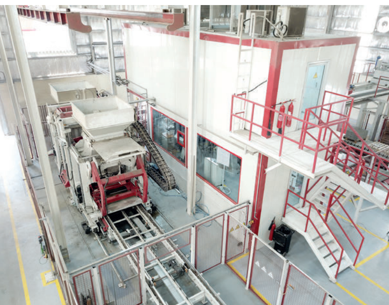
At the heart of the new production line is the Multimat RH 1500-4 concrete block machine.
