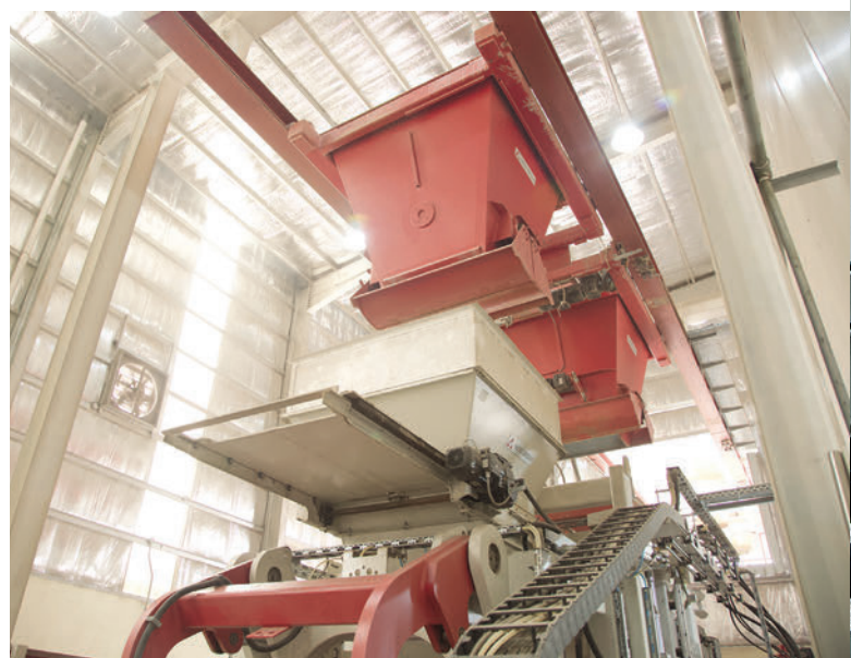
The double bucket conveyor transfers the core and facing concrete into the concrete block machine's corresponding storage silos.
