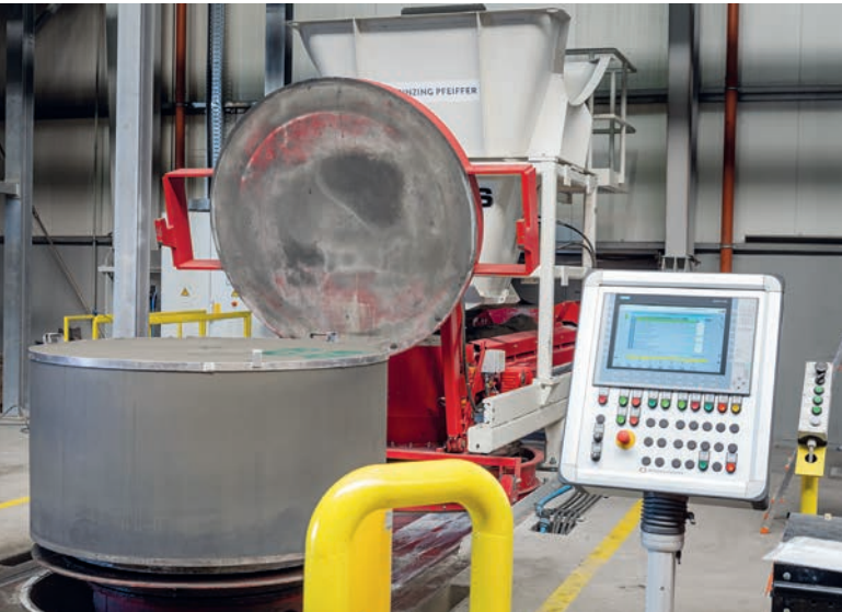
The fresh manhole base element (green base unit) after demoulding
