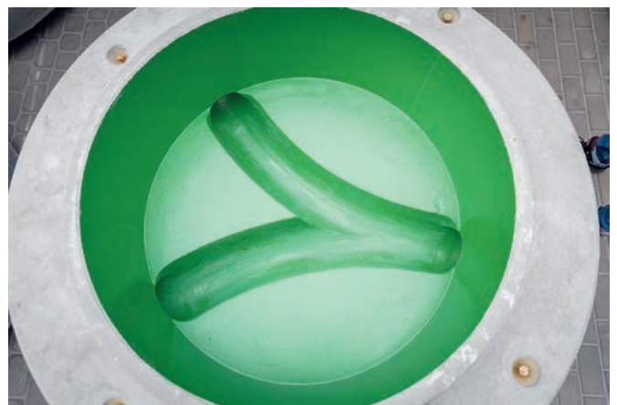
Concrete milling within millimetre accuracy with 2 different milling heads: for inlets and outlets on the left and for the channel on the right
