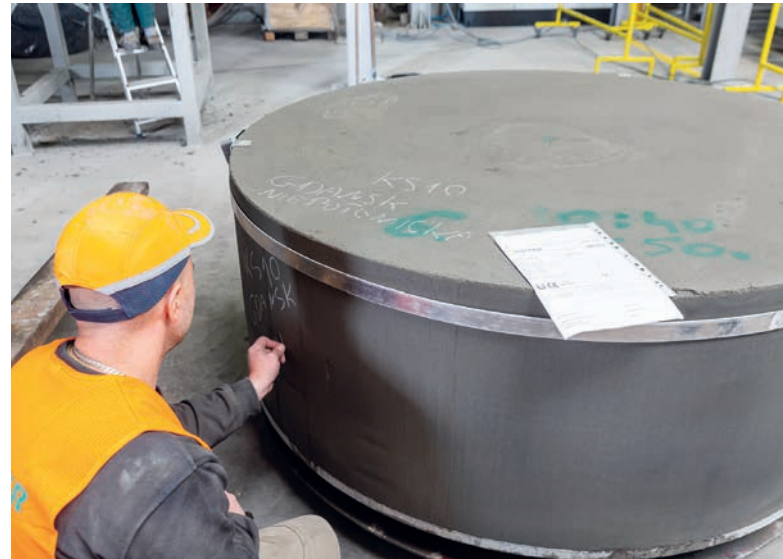
The green base unit is further processed after only 2 hours of curing
