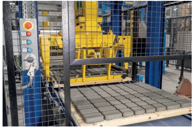
Servo controlled Masa centering device with 4-sided centering clamp
