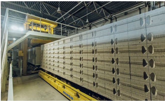
Production of sand lime bricks with the Masa hydraulic press HDP 800
