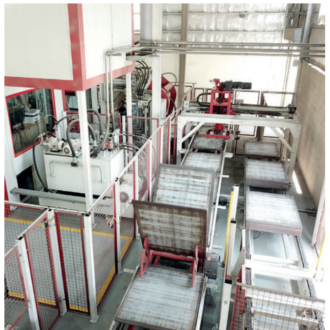
Cross conveyor with board turnover device and board buffer conveyor; in the background the magnetic stacking device
