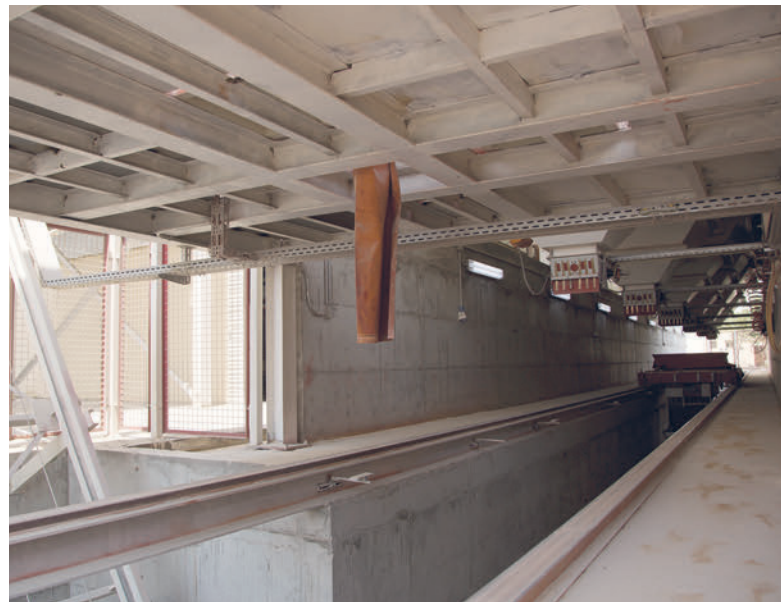
The aggregates are dosed directly from the eight silos arranged in a row. Bucket elevators are responsible for feeding the mixers.
