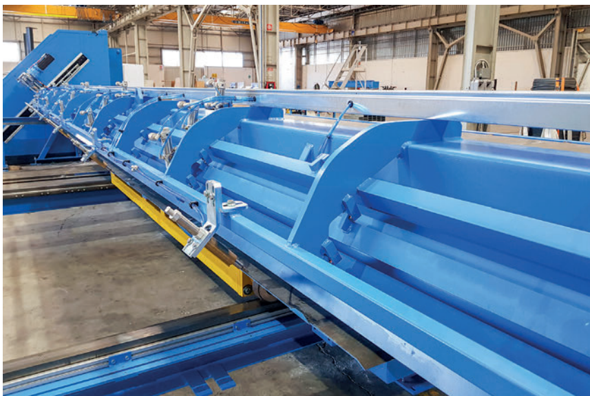
The outlet of the longitudinal bars with 2 outlet flaps and 10 m length catches the cut bars and brings them into position for the likewise automated further transport to welding.
