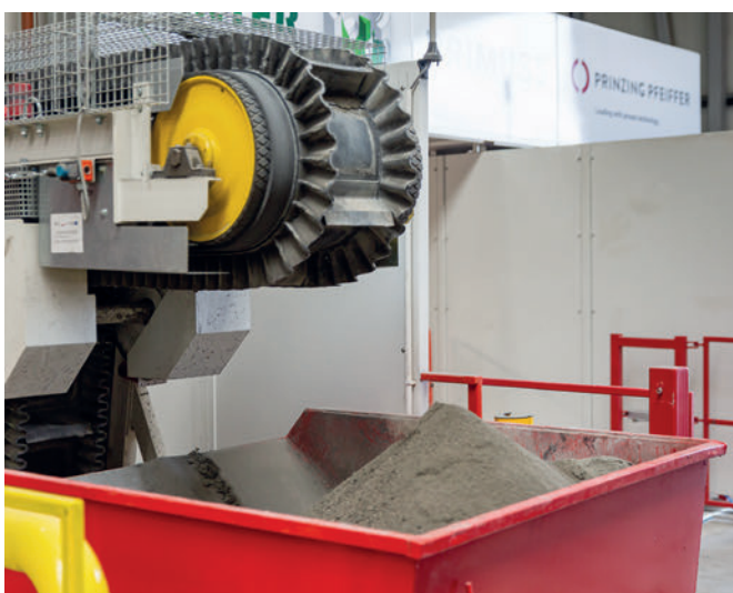
The residual material after milling is conveyed up and can be used again in production
