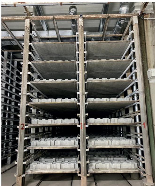
Blocks in the lower part of the rack and blocks in the upper part no longer show any differences in colour.
