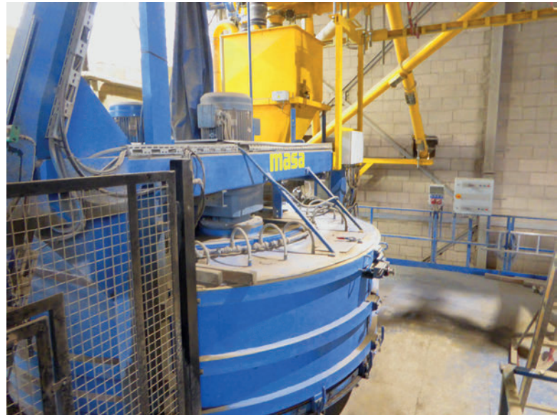
Mixer PH 3000/4500 for main mix concrete
