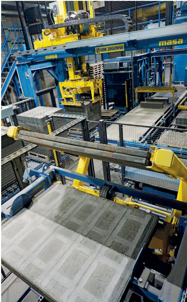
The turnover device (Z type) clamps two production boards each and turns them 180°.
