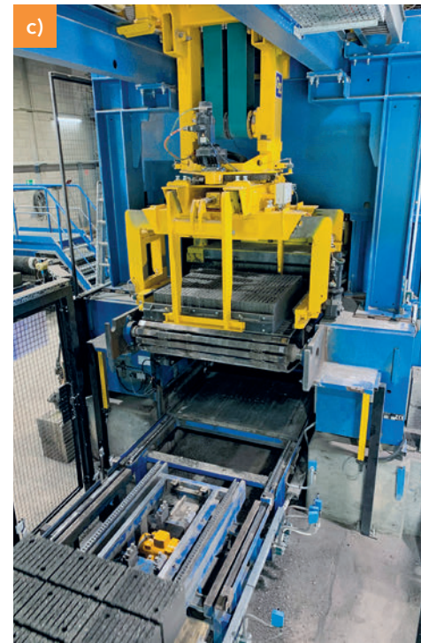
Block loosener and Shifter I: The hardened blocks are loosened from the production board, centered, and gently placed on the feed belt of the grinding system.
