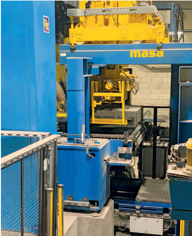
Picking up the grinded products and transferring them in layers onto the return transport.
