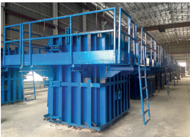
The PBU's are made in a fully automated mould system from Progress Group. They can be filled from above or through the side by a pump system.
