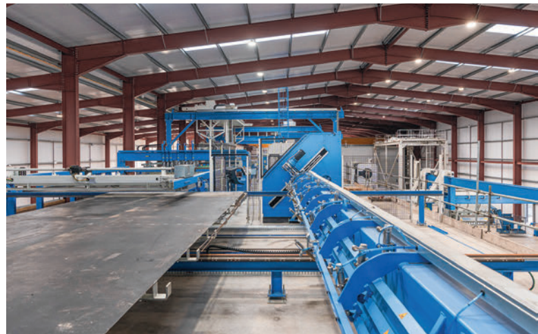
The M-System BlueMesh® mesh welding plant is ensuring a quick production of reinforcement for the precast elements produced.
