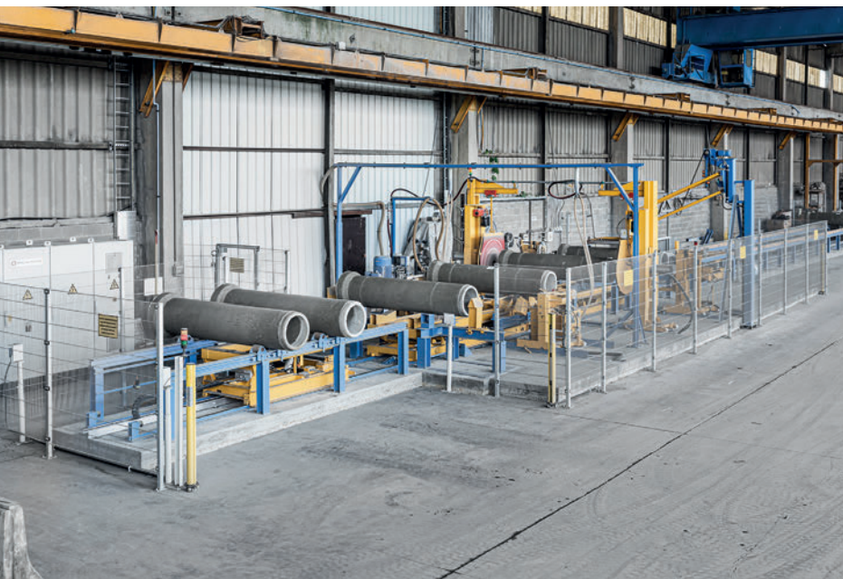
In Beton De Clercq in Gent, Belgium, another concrete plant relies on a pipe testing line from Prinzing Pfeiffer.
