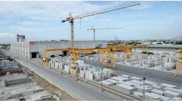
In producing precast concrete elements in factories, the time building on-site is significantly reduced and the quality of the walls and slabs is consistently high.
