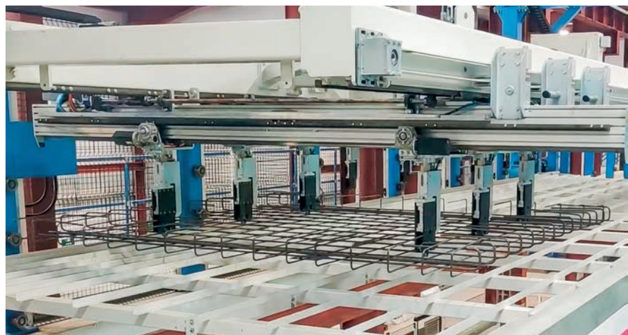
The innovative traverse gripper automates the logistics process even for specially bent mesh and cages
