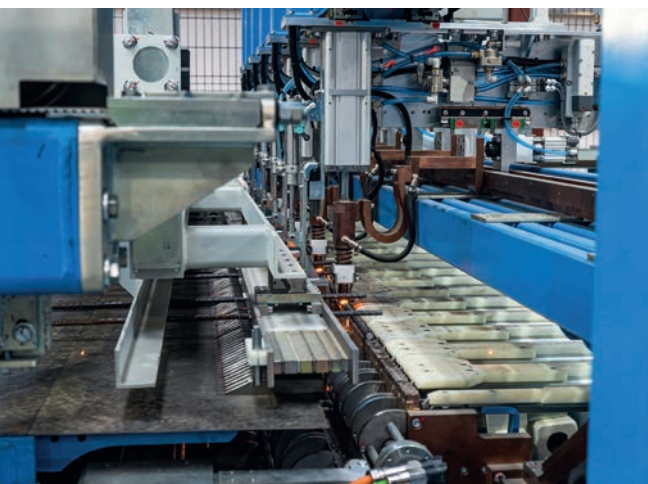
The production of line wire and cross wire without waste - by working directly from coil - without cutting mesh to size, as well as without laying work, also optimises the production flow.
