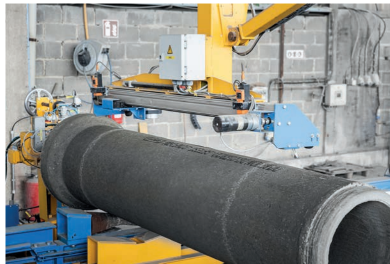
Marking of a tested concrete pipe with the pipe marking device.
