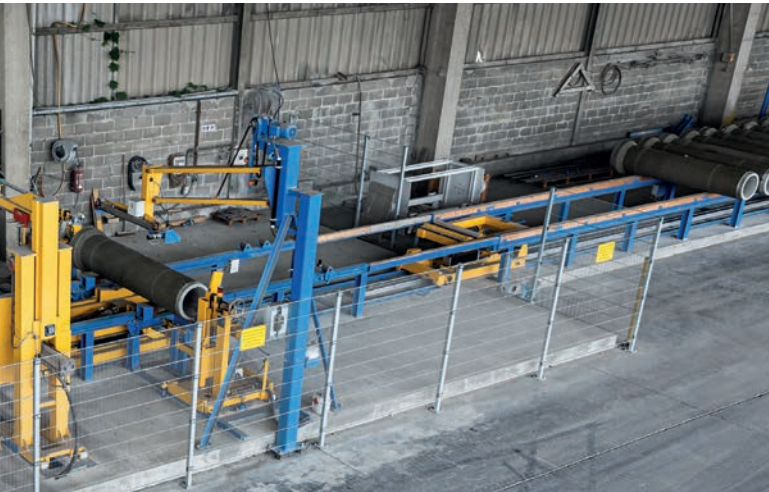
Numerous pipes can be buffered on the pipe deposition track after testing.
