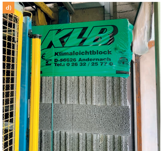
Masa remodeling: The original 10 thermal insulation blocks (16DF KLB SW1 thermal insulation blocks) of the production cycle are reduced to eight blocks to achieve the pallet size.
