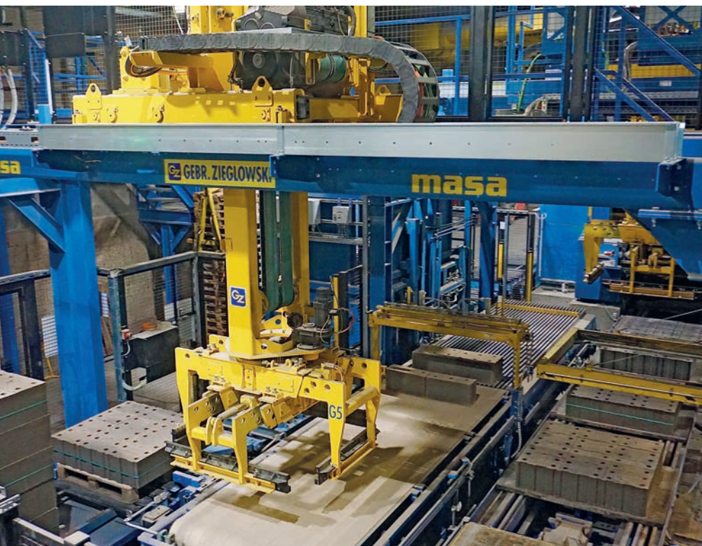
Intelligent interaction of return transport, Shifter, remodeling line and Cuboter
