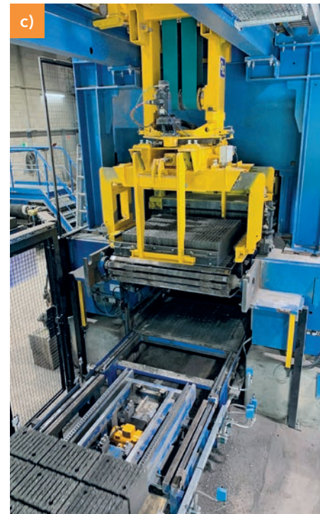
Block loosener and Shifter I: The hardened blocks are loosened from the production board, centered, and gently placed on the feed belt of the grinding system.
