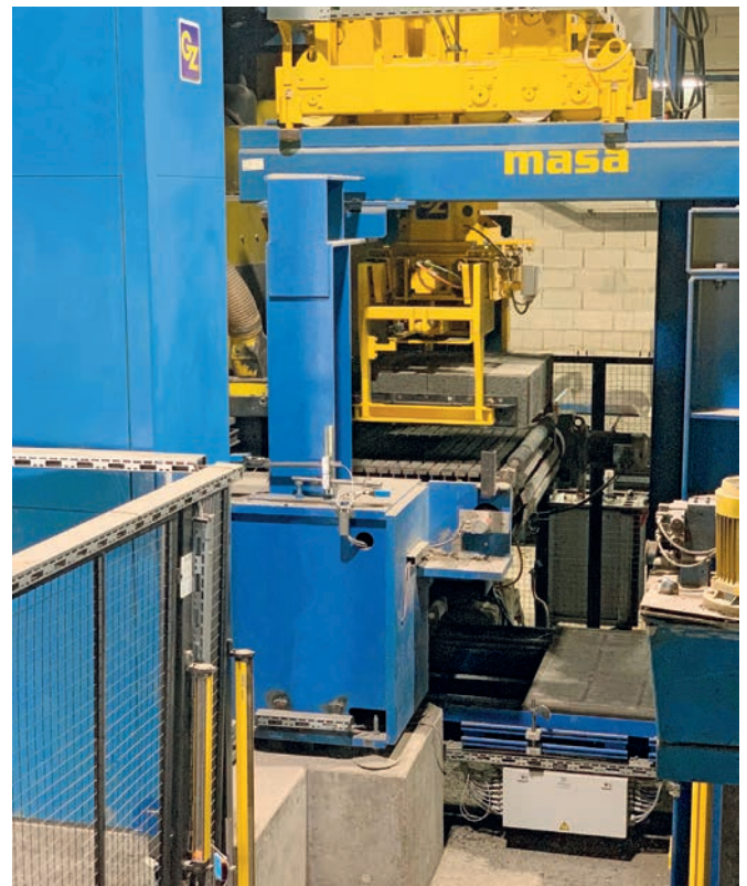
Picking up the grinded products and transferring them in layers onto the return transport.
