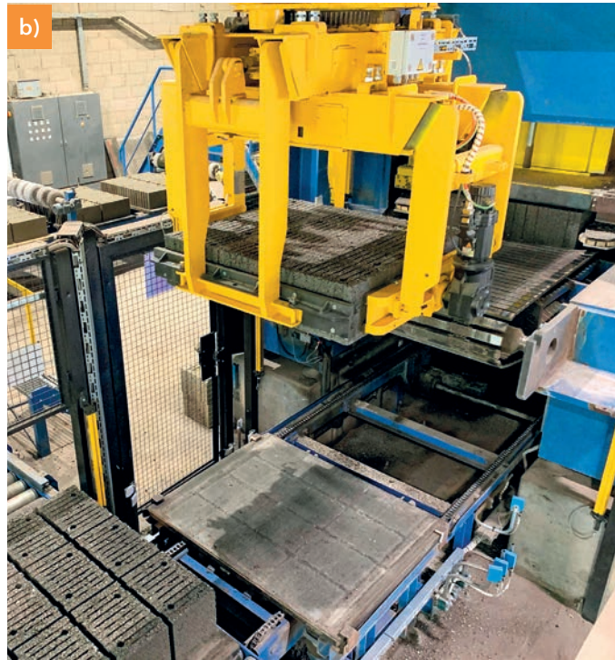
Block loosener and Shifter I: The hardened blocks are loosened from the production board, centered, and gently placed on the feed belt of the grinding system.
