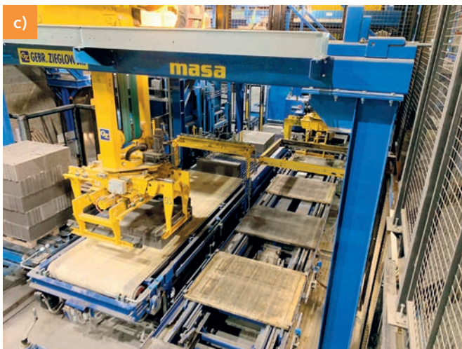
Masa remodeling: The original 10 thermal insulation blocks (16DF KLB SW1 thermal insulation blocks) of the production cycle are reduced to eight blocks to achieve the pallet size.
