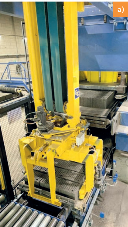
Block loosener and Shifter I: The hardened blocks are loosened from the production board, centered, and gently placed on the feed belt of the grinding system.
