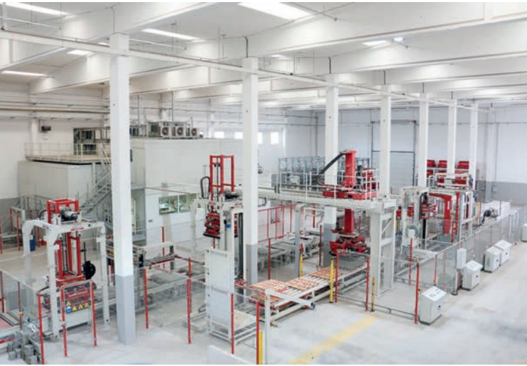
Packaging on the dry side at Siprem: product squeezer, doubler, and cuber
