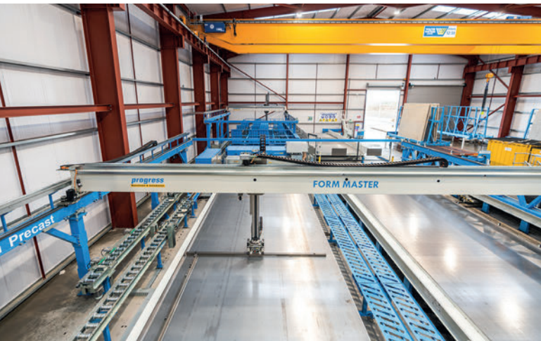
The Form Master shuttering robot places the shutters fully automated and precisely on the pallet surface as well as without any filling elements which would have to be disposed afterwards.
