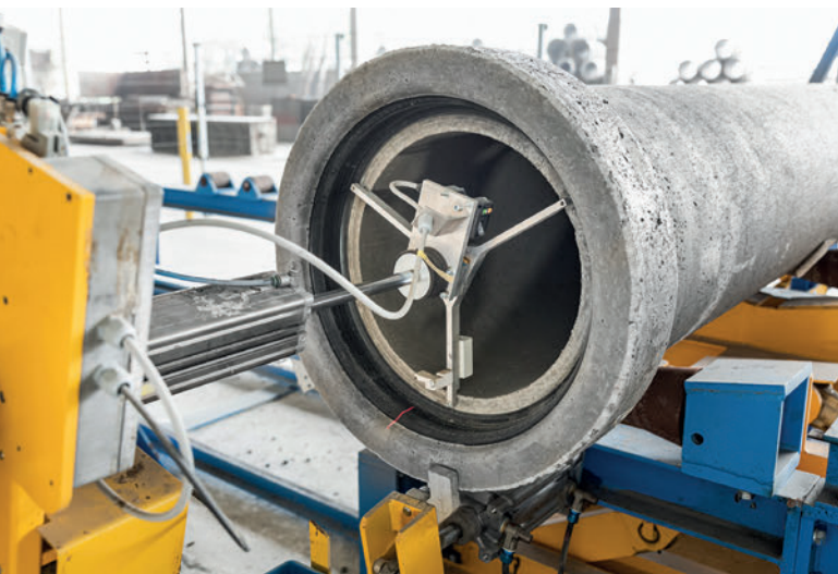
Spigot end, the integrated gasket and straightness measurement in the last station of the test line.
