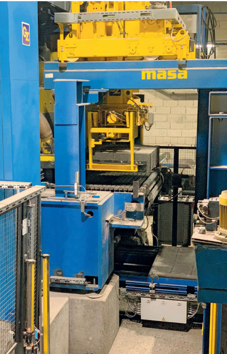
Picking up the grinded products and transferring them in layers onto the return transport.
