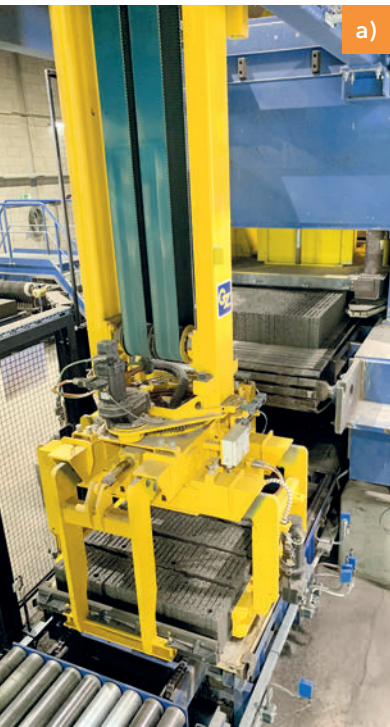
Block loosener and Shifter I: The hardened blocks are loosened from the production board, centered, and gently placed on the feed belt of the grinding system.
