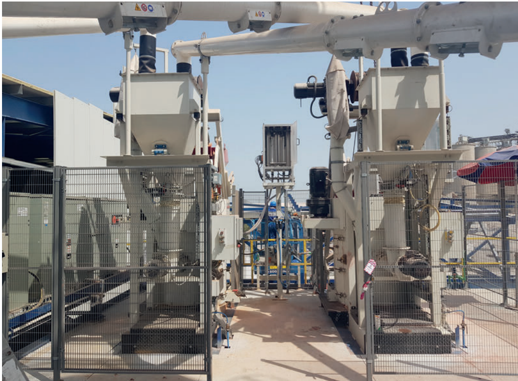
Mixing plant with two face mixers SM 400
