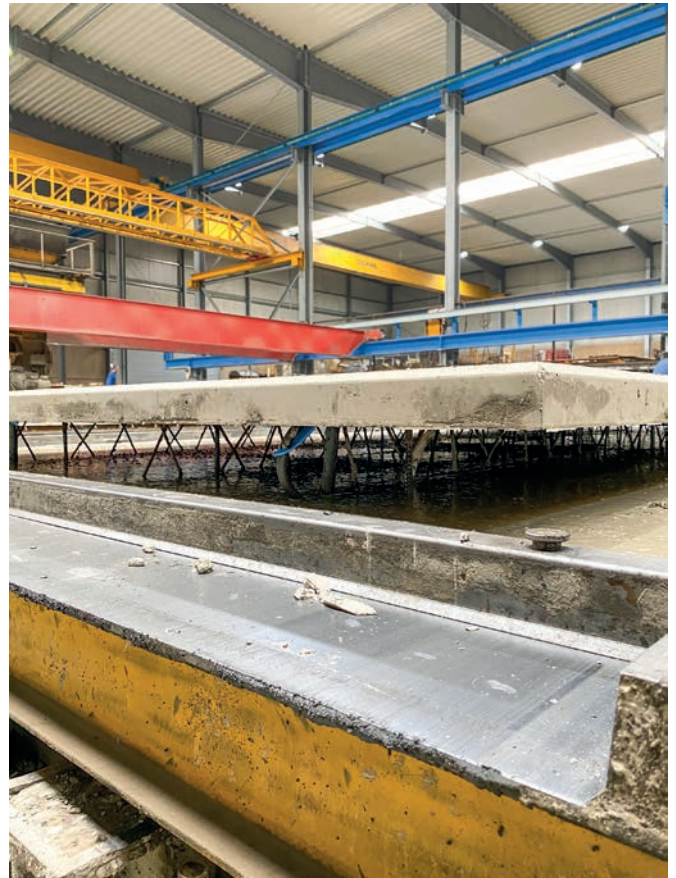
Precast concrete walls and slabs are reinforced with the manufactured lattice girders.
