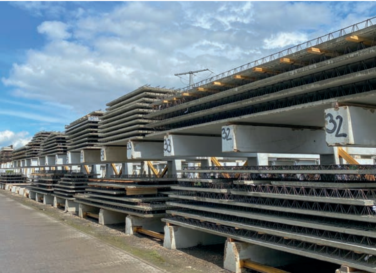
The produced double walls and precast slabs with in-situ topping ready for delivery to the customers.
