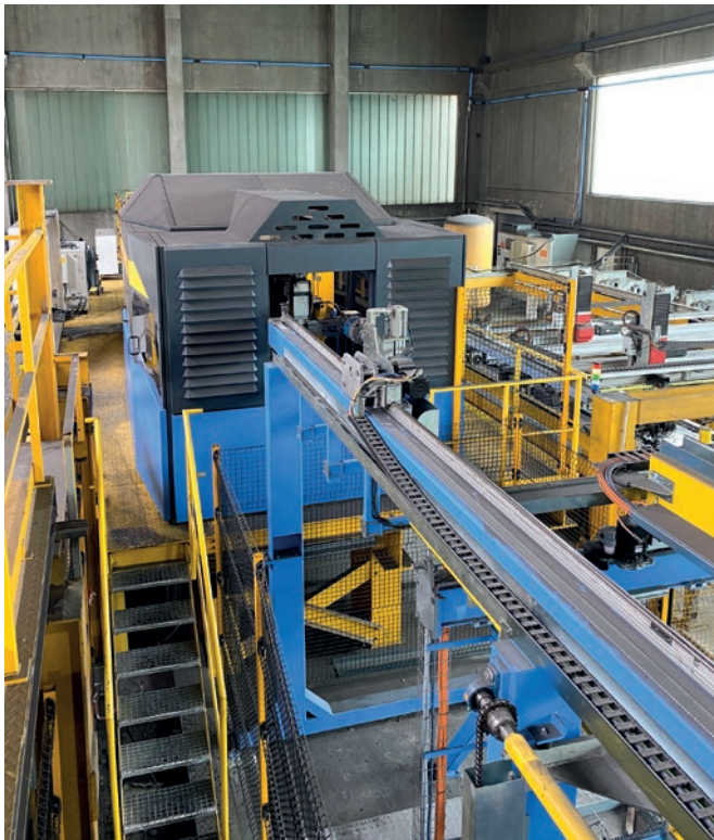
The new fully automatic VGA Versa lattice girder welding machines can switch automatically between girder heights in a very short time and during ongoing production.
