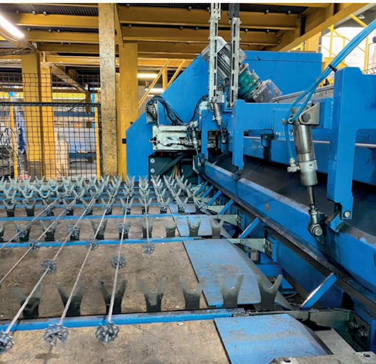
The MSR Multirotor straightening and cutting machine from Progress has an automatic wire diameter changer and is also equipped with an automatic spacer supply.
