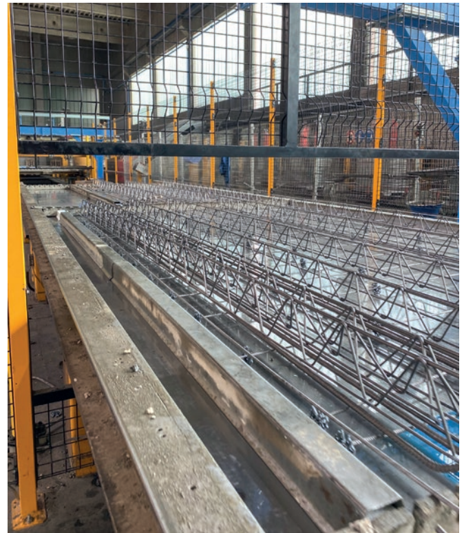
The new fully automatic VGA Versa lattice girder welding machines can switch automatically between girder heights in a very short time and during ongoing production.
