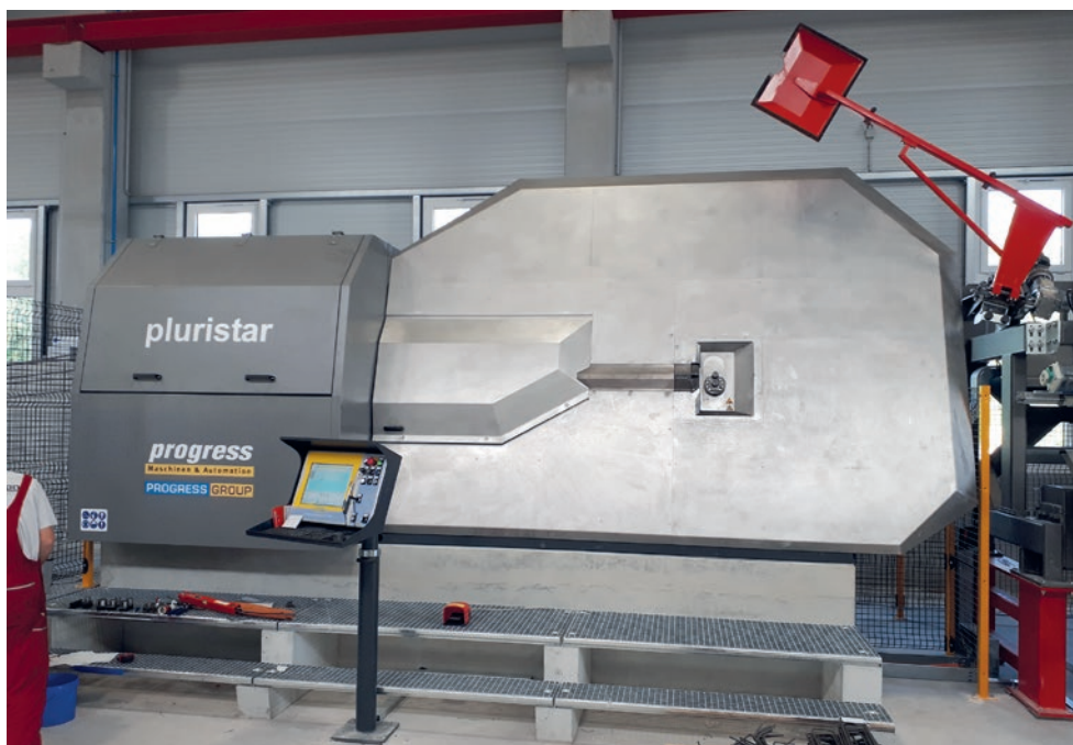
The Pluristar multifunction plant has an automatic changeover from double to single wire processing and an automatic straightening adjustment.
