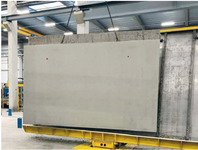
Production of first double walls.
