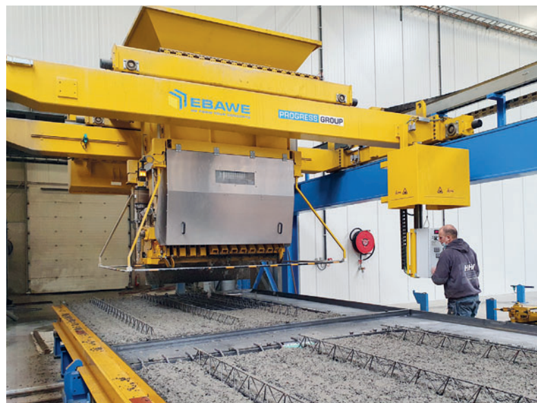
The concrete spreader distributes the fresh concrete into the shuttered pallets, with the made to measure reinforcement already in place.
