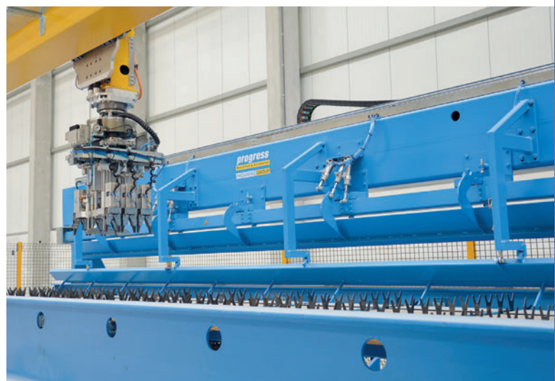
The Wire Center places reinforcement fully automatically and improves production output.
