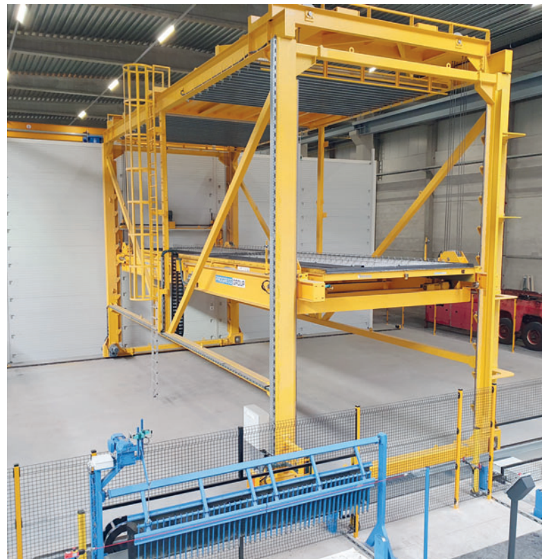
The pallet stacker for stacking and destacking of the pallets fully automated by ebos®
