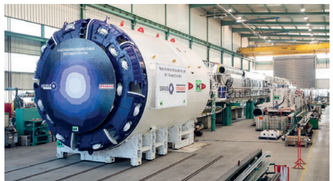
Strabag AG’s S-1175 tunnel boring machine.
