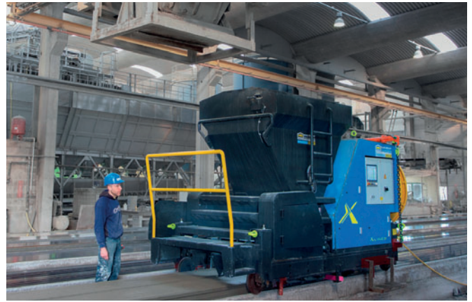
The Extruder X-Liner only needs one machine operator to handle the concrete supply.
