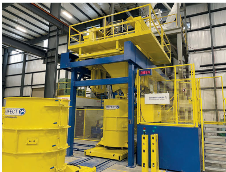
By setting up moulds based on the division of labor, moulds are constantly made available for filling with SCC.
