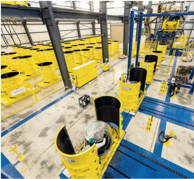
User-friendly moulds and scheduled processes—two cornerstones for efficient precast part manufacturing at Foley
