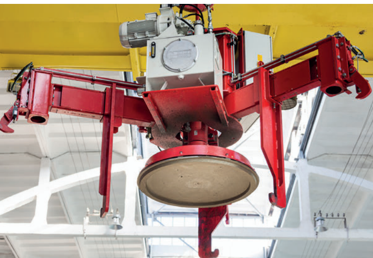
Mobile press/lifting beam of the Atlas 150/150
