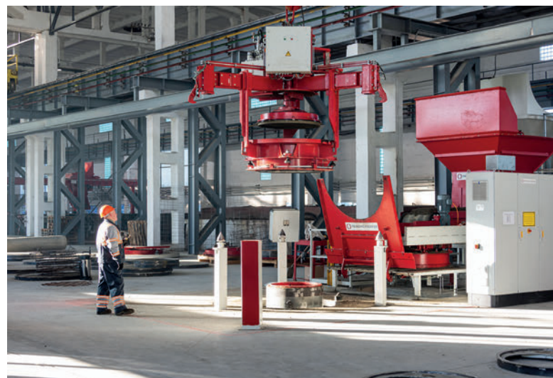
Atlas 150/150 - Manhole cover slab production
