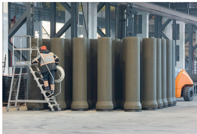
The freshly produced concrete pipes
