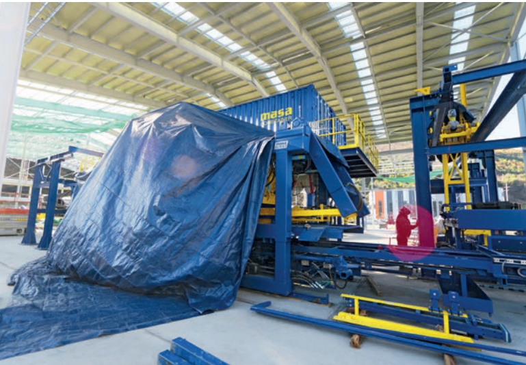
Shrouded: The new Masa XL-R concrete block making machine awaits commissioning.
