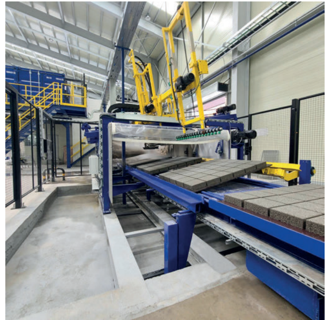
Masa 3-station washing plant: Fine fractions of the aggregates and the cement films are removed by a combined spray and surge process.
