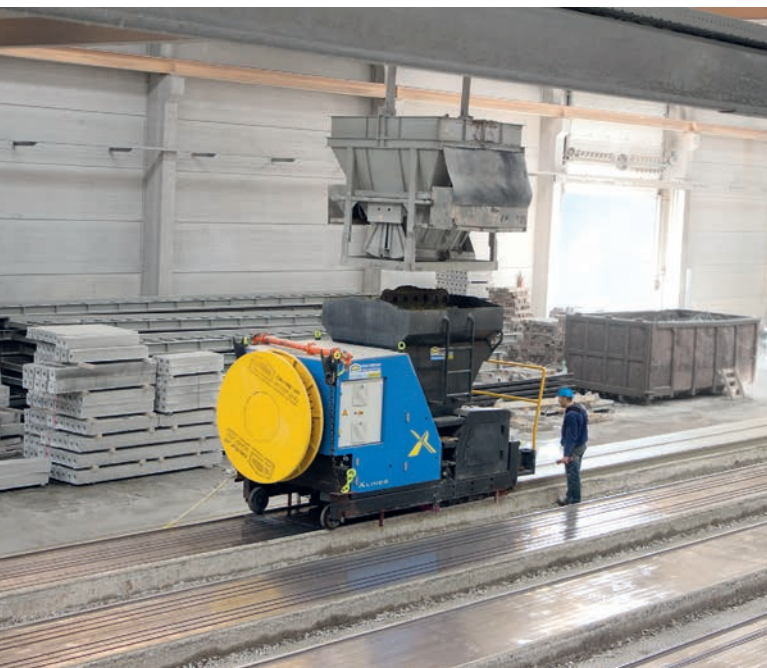
The highly automated production machine Extruder X-Liner FC with "shark screws" guarantee very high compaction.
