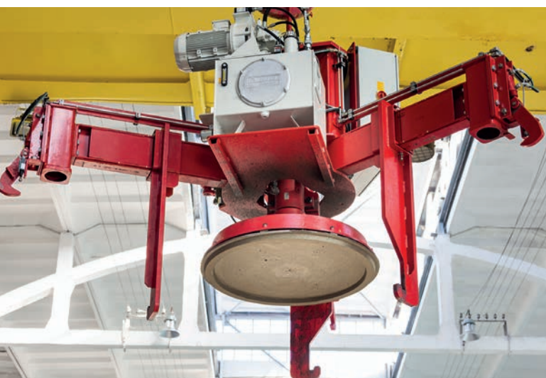
Mobile press/lifting beam of the Atlas 150/150
