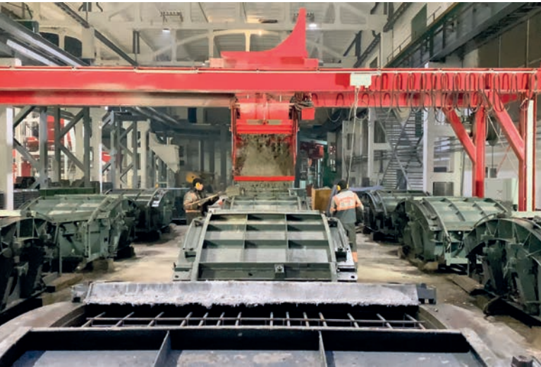
The new concrete distribution system for the tunnel formworks
