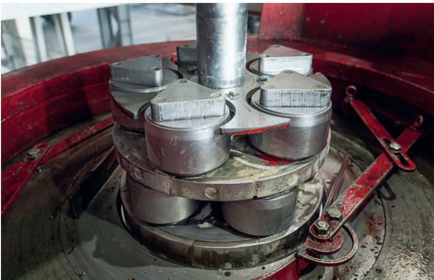
The rollerhead is the compaction tool of the Radial Press / The rollerhead change
