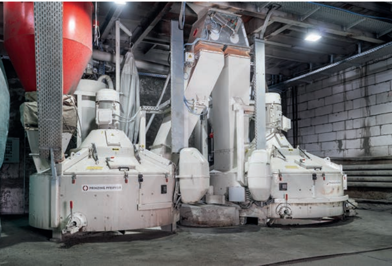
The new SX-series planetary mixers are used to produce concrete mixes for drycast and wetcast processes.
