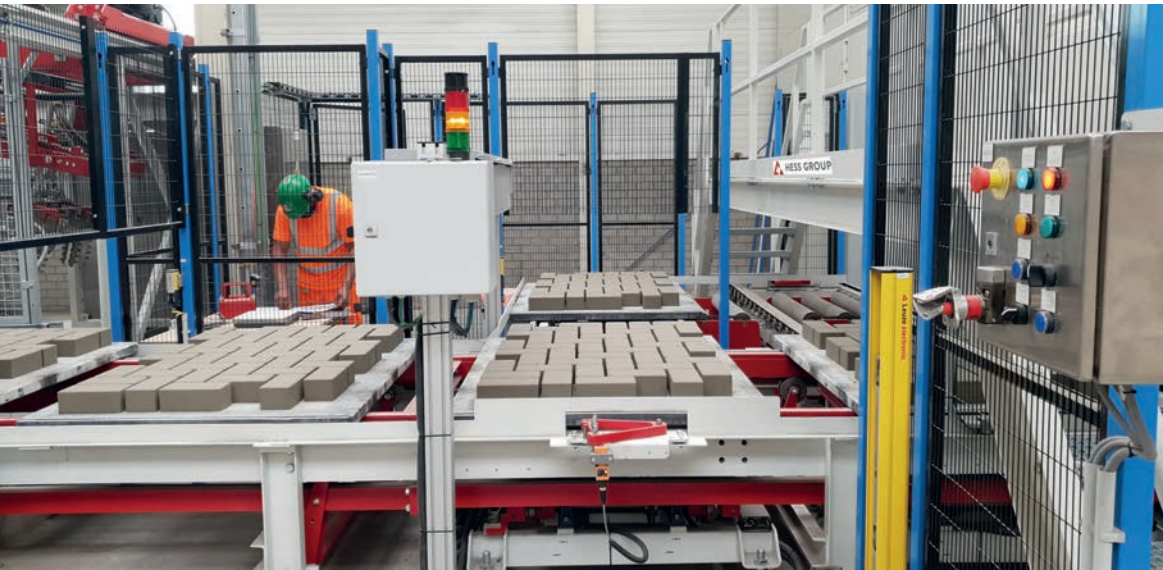
Quality inspection of freshly produced concrete pavers
