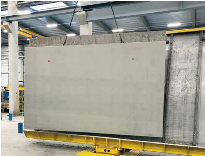
Production of first double walls.
