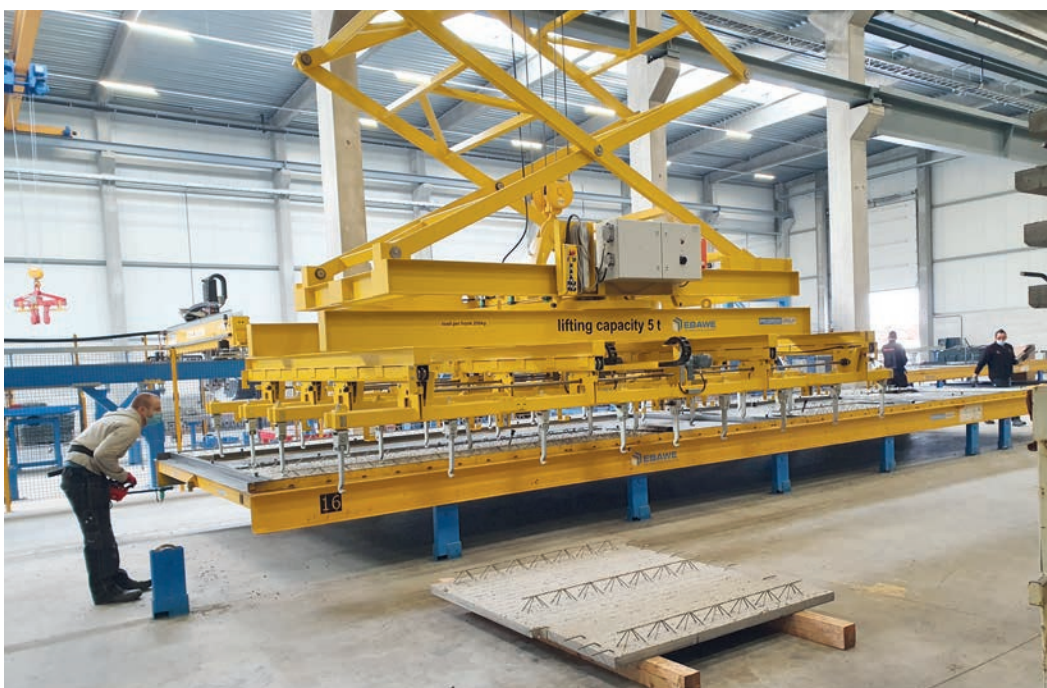
The demoulding crane provides a safe removal of the elements.
