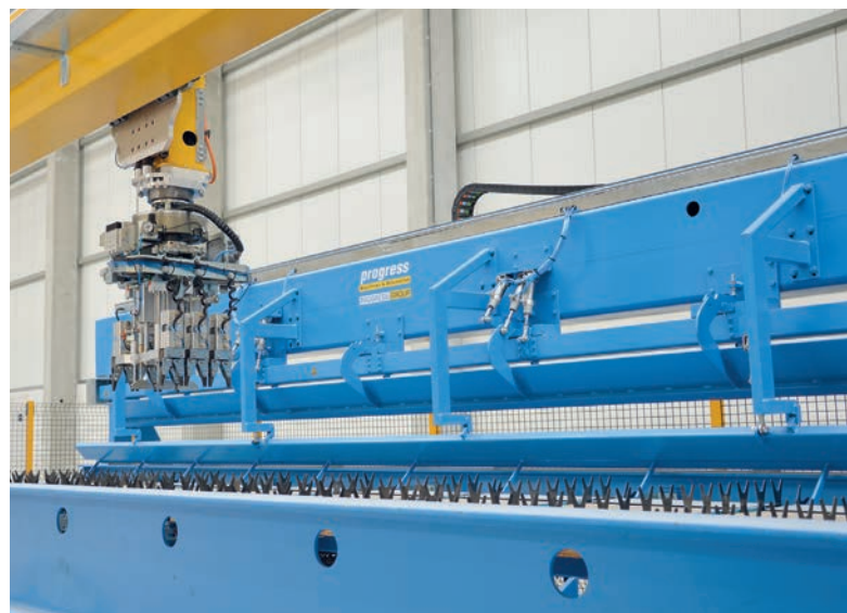
The Wire Center places reinforcement fully automatically and improves production output.
