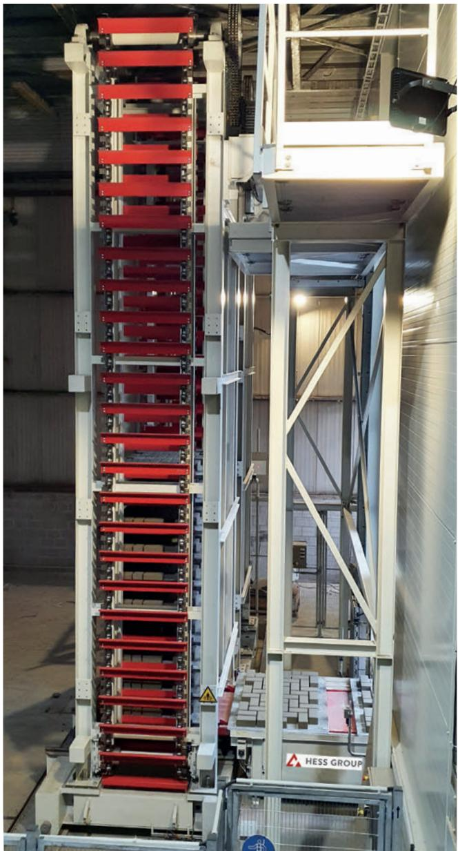
*Elevator system; photo taken from the curing chamber side*
