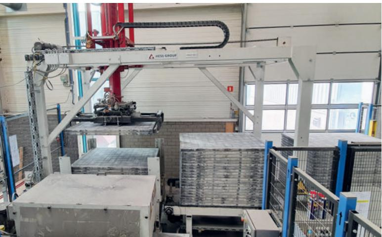
*Production board buffer conveyor with destacking crane and board hopper*
