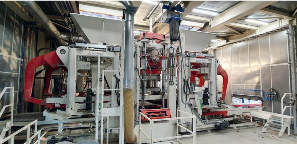
Side view concrete block machine RH 1500-4 MVA
