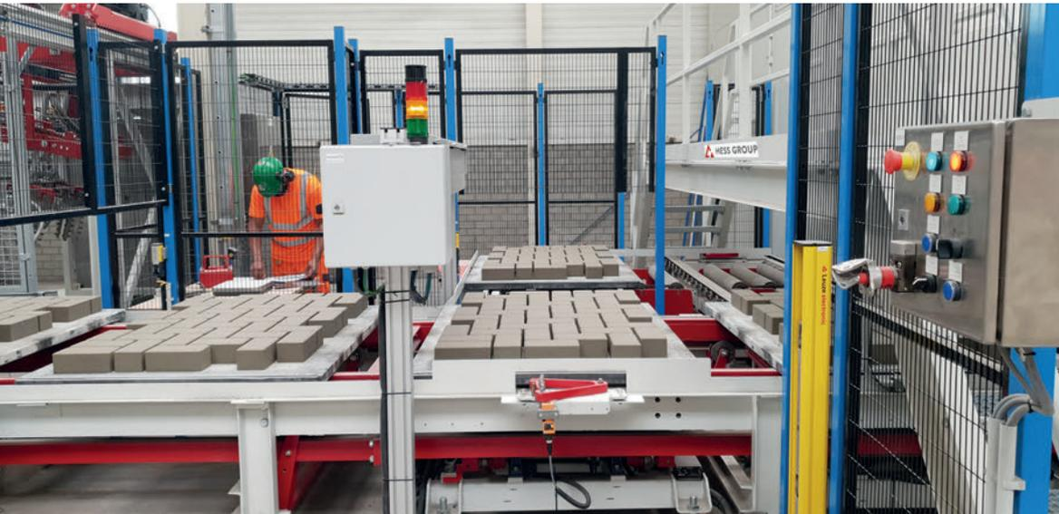
*Quality inspection of freshly produced concrete pavers*
