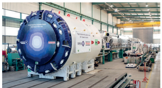
Strabag AG’s S-1175 tunnel boring machine.
