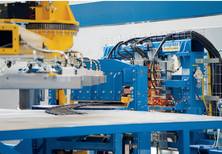
The Tunnel Master uses computerised welding control to produce curved tunnel segments.
