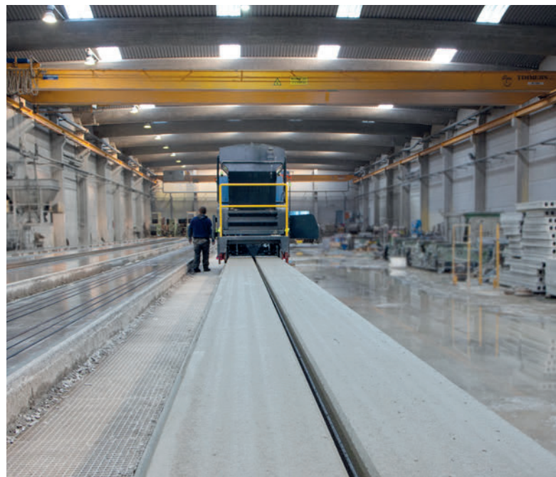
Production bed of 1,2 m, where two hollow core slabs of 60 cm width are being produced at the same time by an Extruder X-Liner
