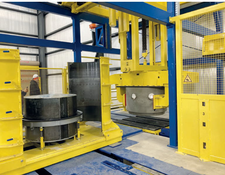
Automated manhole base demoulding with optimized cycle time
