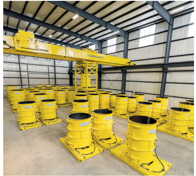
Reduction of costs and risks through automated mould management in the hardening area
