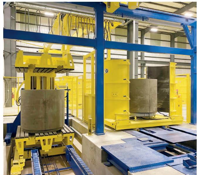
When required, demoulded products are automatically and carefully rotated by 180 degrees.
