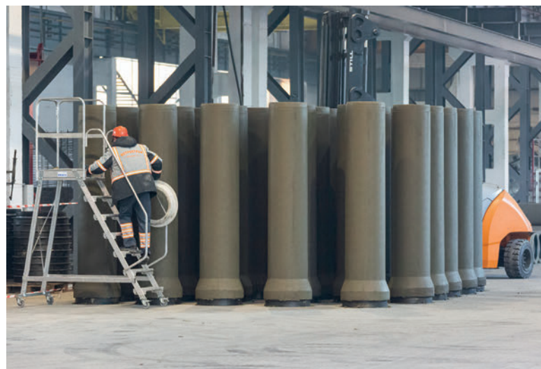
The freshly produced concrete pipes
