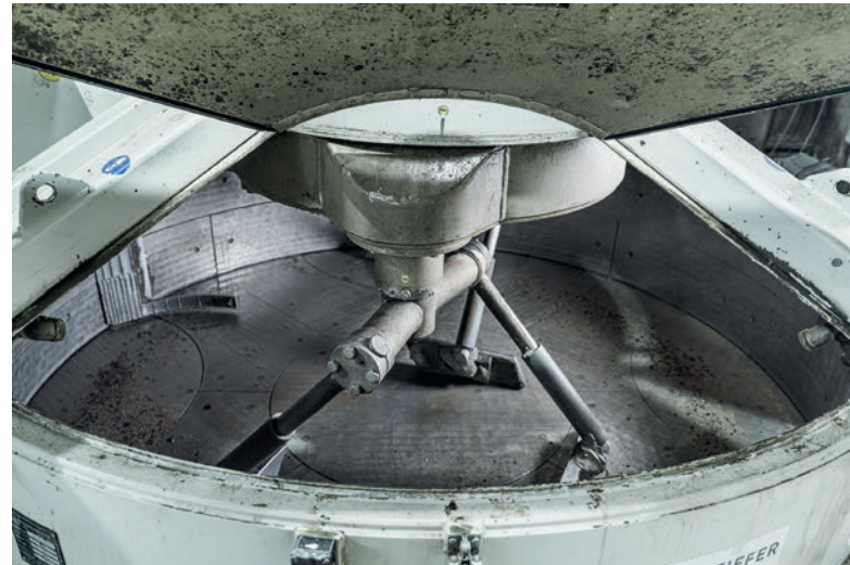
Large maintenance flaps make the mixer easily accessible.
