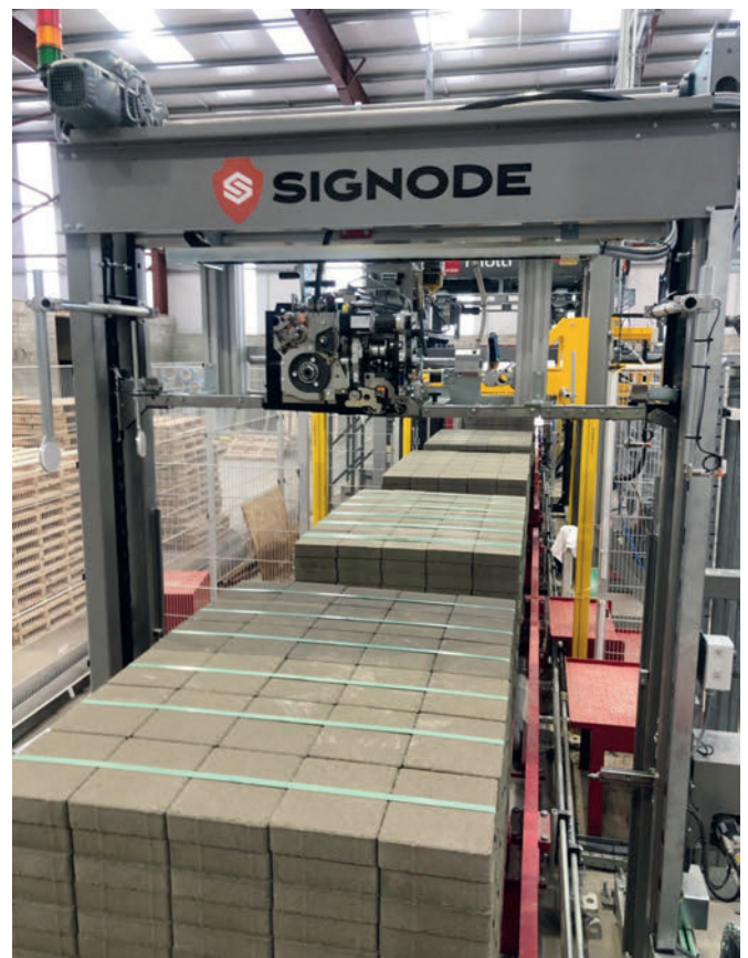
Strapping is performed on a TSM-H6500 machine with Jumbo Reel Dispenser and HSM-H3000 head from manufacturer Signode.
