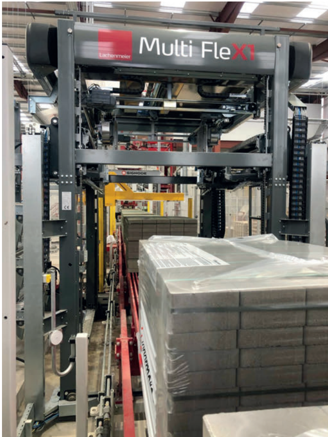
After strapping, a Multi FleX1 stretch hooding machine from Lachenmeier covers the stabilized packs with a stretch hood.
