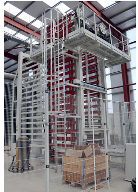
There is one buffer car behind the elevator and one in front of the lowerator on the wet side and on the dry side respectively, each with 17 tiers (double discharge system) and 14 tons of capacity.
