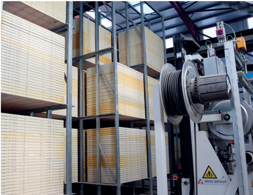
Buffer with 3,240 production pallets at the beginning of the wet side.
