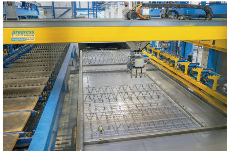
The Wire Center installs transverse reinforcement with and without spacers as well as longitudinal reinforcement and lattice girders according to CAD specifications.
