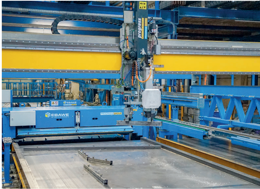
The demoulding robot removes the formwork fully automatically before the pallet is forwarded to the cleaning device.
