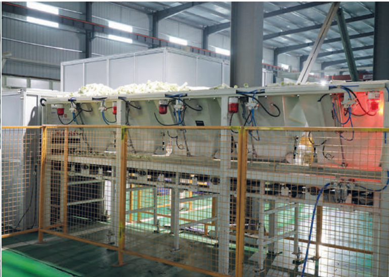
Figure 10: Feeding system for screw anchors to be installed automatically by robots
