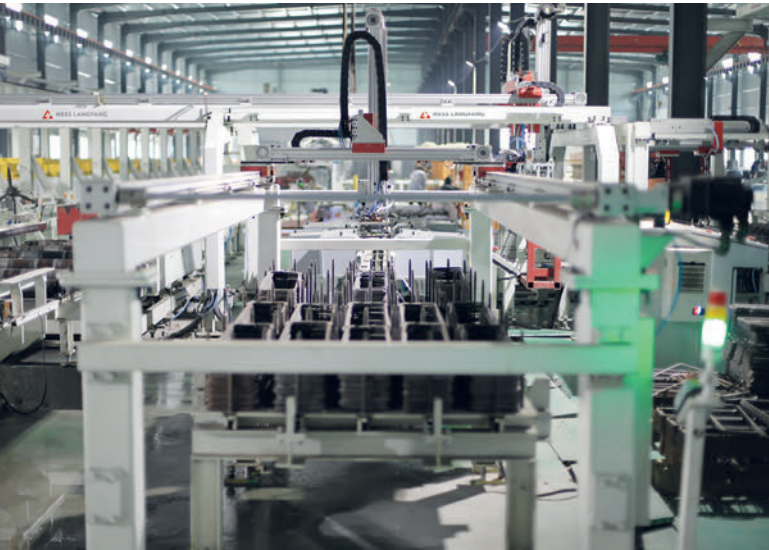
Figure 7: Automated railway sleeper steel reinforcement installation station
