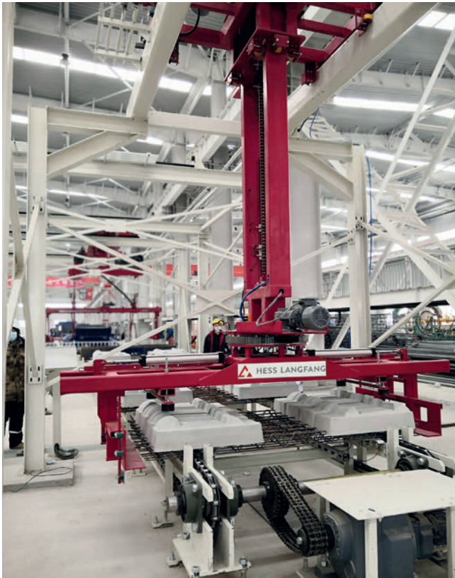
Figure 6: Automated sleepers stacking device
