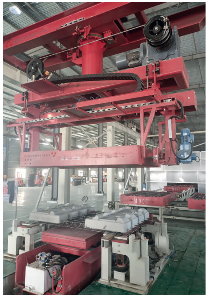
Figure 5: De-molding system with mold turning device and demolding table
