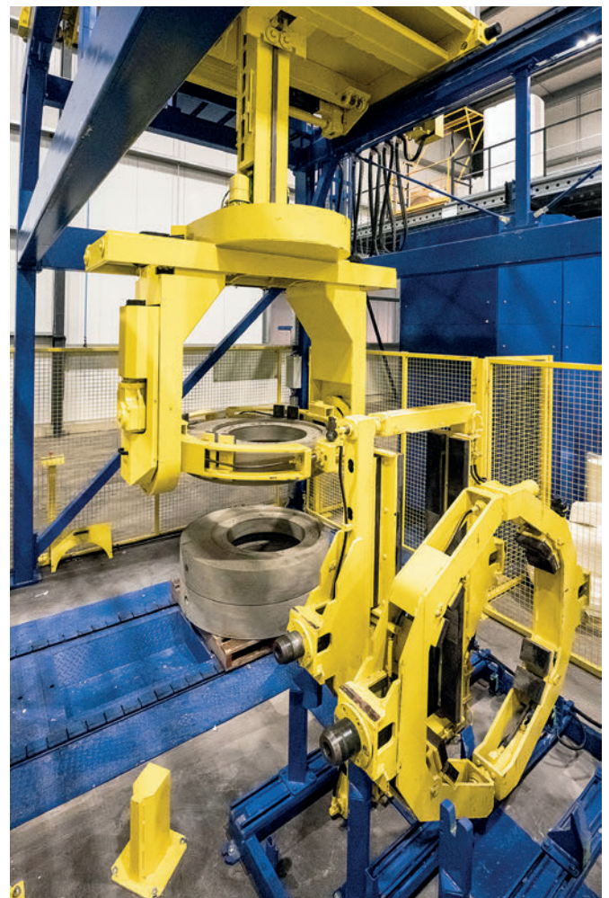
The automatic product manipulator gently removes the products from the moulds.
