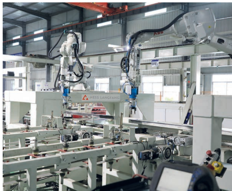
Figure 9: Robots screwing-in spring elements into the railway sleeper molds - fully automated
