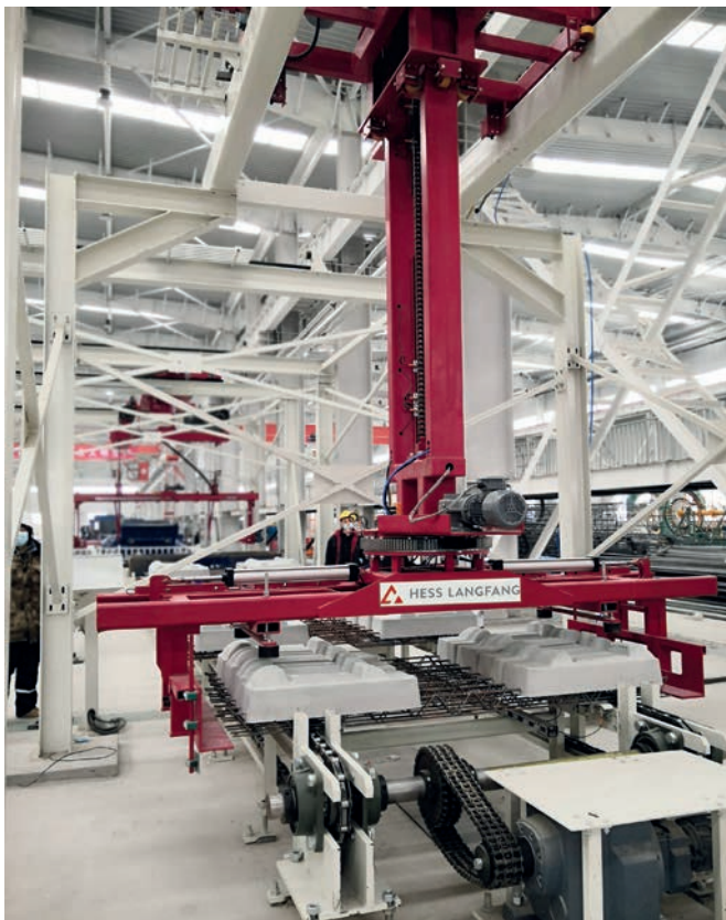
Figure 6: Automated sleepers stacking device
