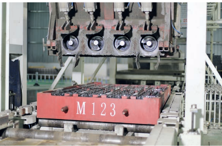
Figure 3: Automated casting and vibration station
