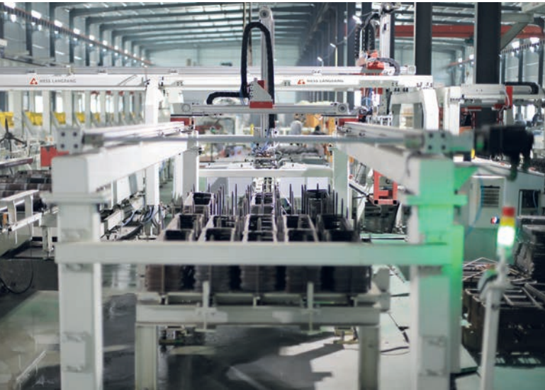
Figure 7: Automated railway sleeper steel reinforcement installation station
