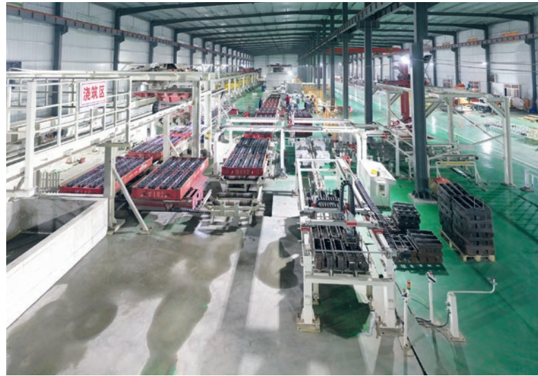
Figure 12: Fully automated installation of embedded parts / steel reinforcement
