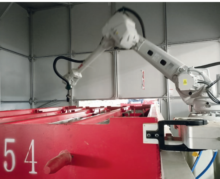
Figure 13: Mold spraying of release agent by robots
