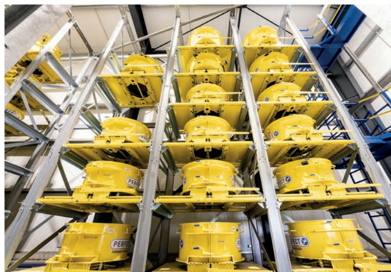
An efficient way of storing the mould-hardened product and making use of the energy released by the concrete during hardening.
