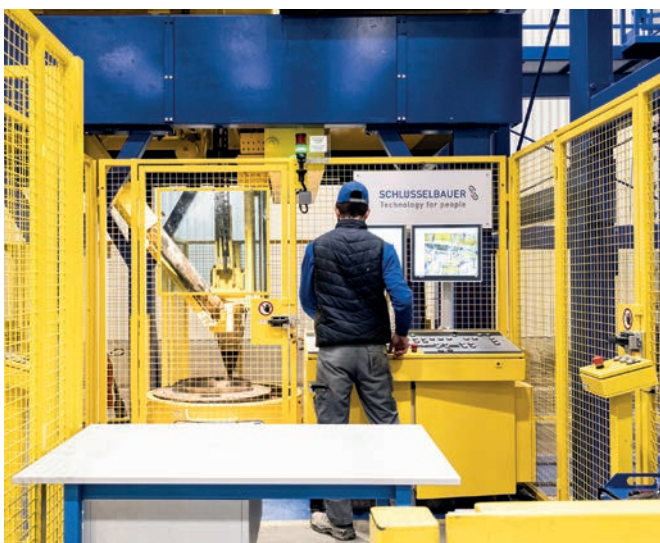
The operator monitors the filling process and the storage and retrieval of moulds in the high-bay racks from a central operating panel.
