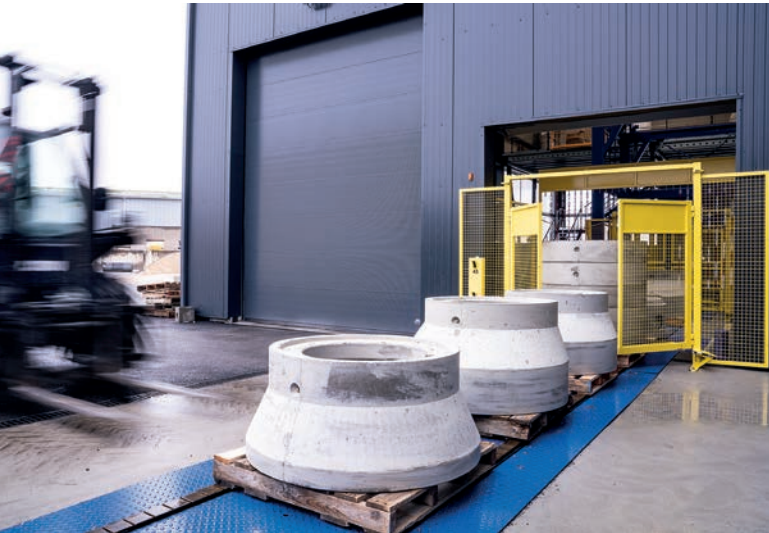
The demoulded manhole parts leave the building on pallets ready for loading.
