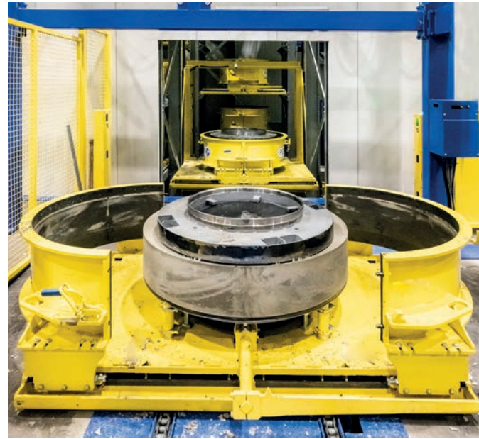
One mould after another is removed from the high-bay racks.
