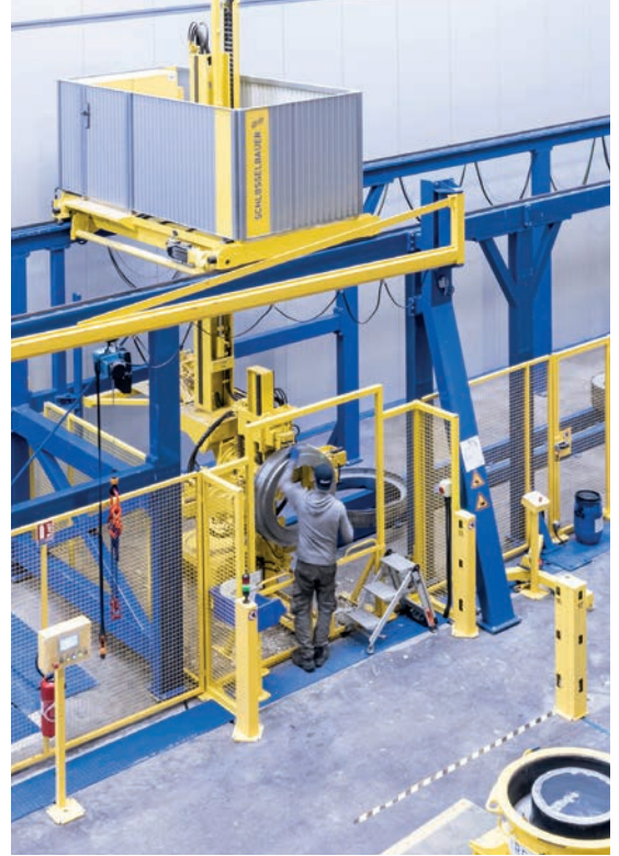
Top pallets are automatically transported to an ergonomically optimized workplace for cleaning.
